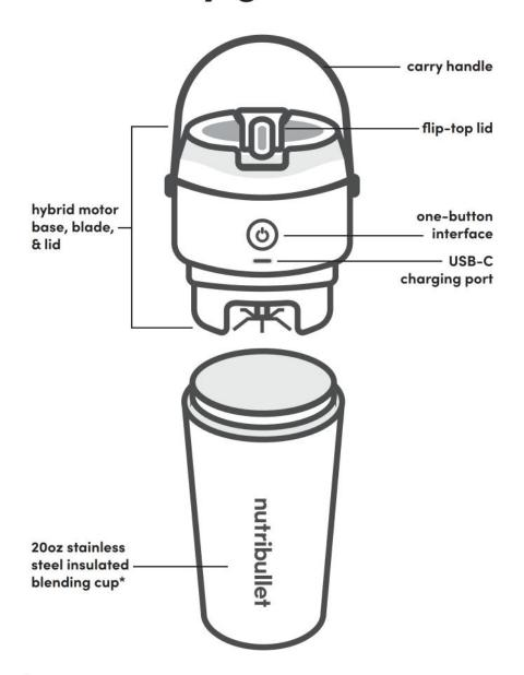
\*WARNING! DO NOT exceed the MAX fill capacity. 20oz total Cup capacity. 16oz MAX fill line capacity.
