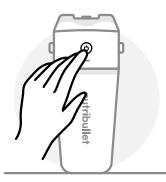
4 With the blender right side-up (Hybrid Motor Base, Blade, and Lid on top), press the Power Button once to wake up the blender. Wait about 1 second for the LED light ring to fully illuminate.
