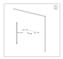
Connct the mirror wires with your main wires and hang the mounting hole to the screw on the wall.
