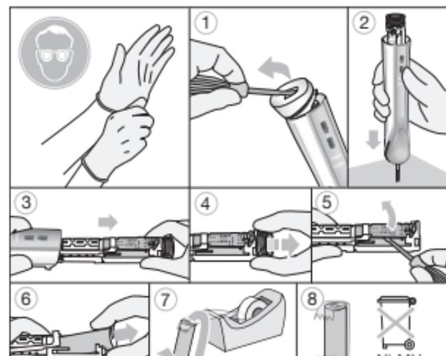
Open the handle as shown, remove the battery and dispose of it according to local environmental regulations. Caution! Opening the handle will destroy the appliance and invalidate the warranty.
