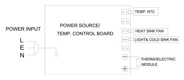
• The inside temperature of the thermoelectric wine cooler depends on the room temperature. The wine cooler can be adjusted in the range of  $8^{\circ}$ — $18^{\circ}$ C (±  $1^{\circ}$ C), when it is located in an ideal room temperature of 25°C.By first time turn on, without putting any bottle inside the wine cooler, the product can be cooled to  $15^{\circ}$ C after 1.5 hours and after 2~2.5 hours more will reach to the temperature programmed by the manufacturer.
