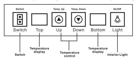
The temperature range for Wine Cooler is Top 12-18°C / Bottom 8-18°C. When the temperature is set on one certain point and the temperature inside reaches this point, the automatic temperature control system begins to work and the cooling system goes into linear temperature keeping status.
