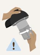
**Good to know:** Notice the direction of the lock icon arrow printed on the filter basket. The basket should be the only part turning when locking and unlocking. It does **not** click, but the basket should fit snuggly against the top.
