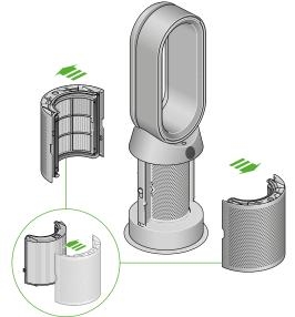
The air purifier fan heater with the filter covers open showing a HEPA plus carbon filter located in the filter covers. Arrows demonstrate that the filter covers will need to be assembled onto the base of the machine.
