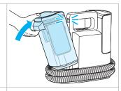
6. Place cap onto tank and tighten. Align tank with machine and press down until it clicks into place.
