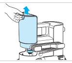
2. Remove clean tank by gripping handle and lifting up.
