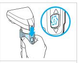
**6.** Slide tool lever up to ensure tool is in SPRAY mode. Follow steps 4-6 above to clean.
