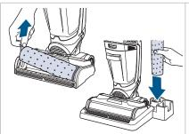
**1.** Remove brush roll following steps on page 3. Pull brush roll tab and place in tray to dry. Check steam bar for clogs. Wipe steam nozzle with cloth.
