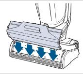
5. Replace the brush roll window by lining up tabs on the edges of the foot.
