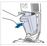
**9.** Insert bottom of tank first. Pivot top toward the machine until it clicks.
