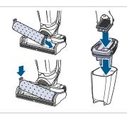
**8.** Reinstall brush roll following steps on page 3. Reinstall filter, strainer, and tank lid.
