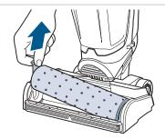
2. Remove the brush roll by pulling the tab.
