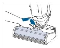
**1.** Grab the front of the brush window and pull upward to remove.
