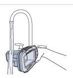
**6.** Rinse the bottom of the tank cover to remove wet debris.
