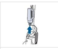
1. The clean water tank is located on the back of the machine. To remove, grasp the tank and pull up.
