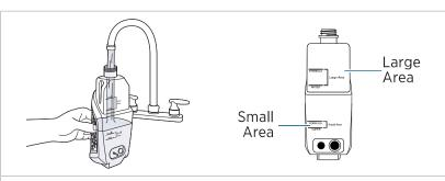
4. The clean water tank has a Large Area volume and a Small Area volume. Pick the one that best suits the space that you would like to clean.
