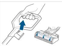
4. Before each use, hold solution spray trigger for 10 seconds to wet the brush roll. **Note:** Bubbles will appear in brush roll window when solution is flowing. Water on floor during steam cleaning is normal.
