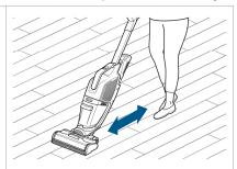
3. With trigger released, make forward and backward passes to extract solution.
