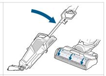
**3.** Recline machine to start brush roll spinning. When machine is standing upright, brush roll will not spin.
