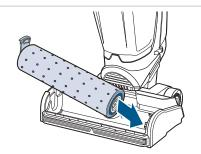
3. Reinstall by placing the end of the brush into the right side of the foot.
