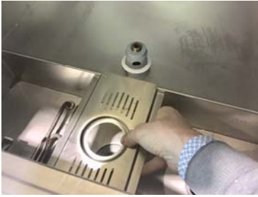
After the cleaning replace all components in the machine. Insert the central support
