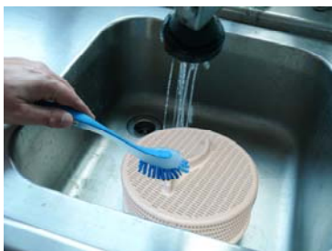
Clean the pump inlet filter by means of a brush
