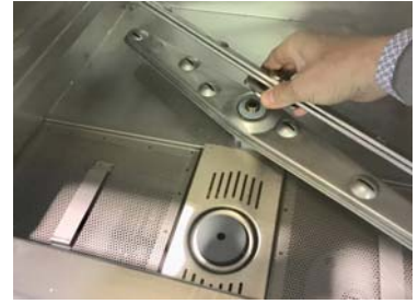
Replace the lower rinse arm
