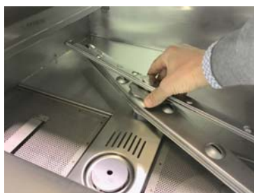
Unscrew the lower rinse arm
