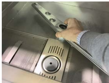
Replace the lower washing arm
