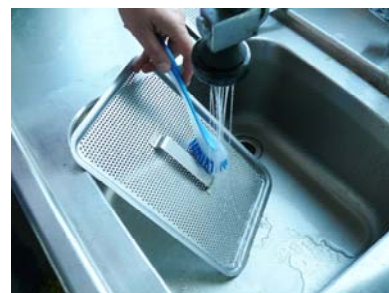
Clean the filter tank top
