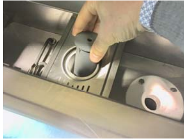
Insert the overflow
