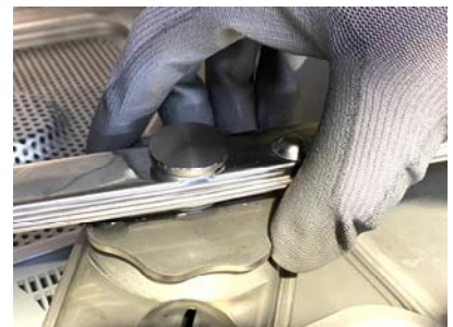
ATTENTION! Daily disassemble the lower rinse arms by working on the „big“ ring nut, like in the picture.
