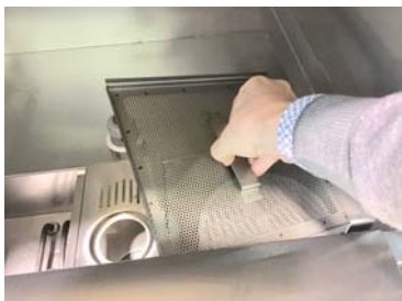
Remove the tank filters on the right
