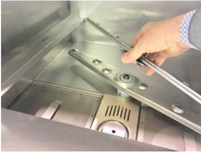
Remove the lower rinse arm
