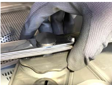
ATTENTION! Daily assemble the lower rinse arms by working on the „big“ ring nut, like in the picture.
