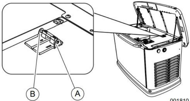
**Figure 2-9. Generator Main Line Circuit Breaker**
