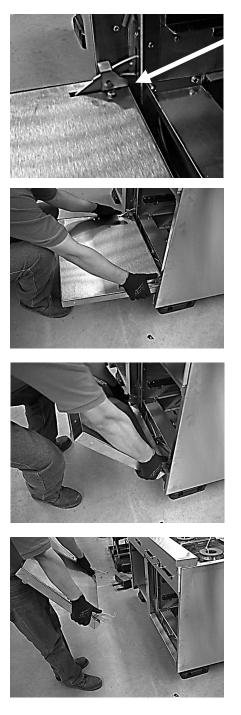
STEP 1.- Place in this way the assembler component in both hinges (you can find 2 pieces of it in carton legs box)
