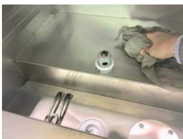
Wipe with a cloth the tank and check for any debris on the bottom.
