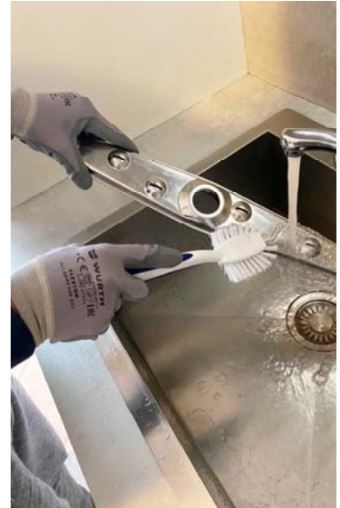
Clean the washing arm for any debris inside.
