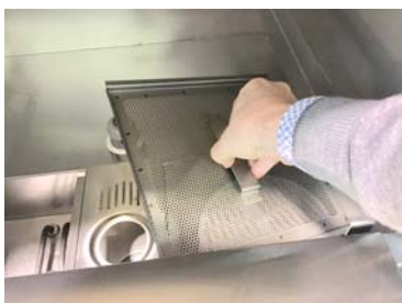
Remove the tank filters on the right
