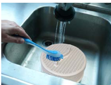
Clean the pump inlet filter by means of a brush
